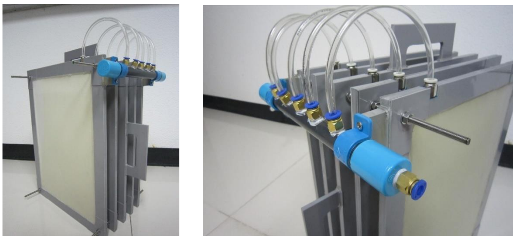
Figure 2.20 Second stage membrane flat sheet design (Vongsayalath, 2015)
