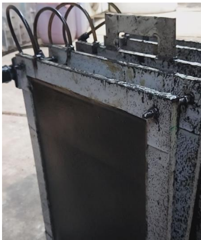
After operation- Fouled membrane
